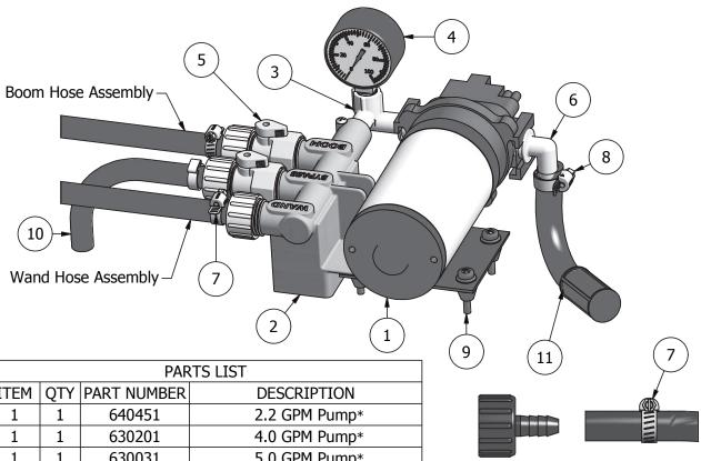
**ITEM** 5.0 GPM Pump\* Manifold Body Elbow (2.2 pumps) Elbow (4.0 & 5.0 pumps) Gauge 0-100 PSI Inline Valve QD EL 12 5/8" Hose Clamp 1/2" Hose Clamp 10-24 x 1.25 Screw Relief Hose Assembly Suction Hose Assembly Cap Assembly (not shown)
